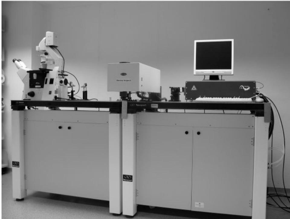
Fig. 2. The multiphoton tomograph DermalInspect and the multiphoton fluorescence lifetime microscope \tau -map.
